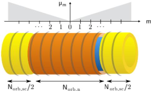
$$\begin{aligned} H = & H_{\text{int},\uparrow} + H_{\text{int},\downarrow} && \rightarrow 1/3\uparrow \otimes -1/3\downarrow \\ & + \sum_{m,\sigma} \mu_m c_{m,\sigma}^\dagger c_{m,\sigma} && \rightarrow \text{confining potential} \\ & + \frac{1}{2C} (\hat{N} - \hat{N}_0)^2 && \rightarrow \text{charging energy} \\ & + \Delta_0 \sum_m f_m c_{m,\uparrow}^\dagger c_{m,\downarrow}^\dagger + h.c && \rightarrow s\text{-wave pairing} \end{aligned}$$
